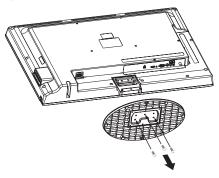
**3** Remove the screws what secure the stand column to the TV, then remove the column.
